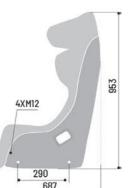
HOMOLOGATION: FIA 8862-2009 MATERIAL: CARBON FIBER HRS: YES WEIGHT (GR): SHELL: 7500 / SEAT: 10750
