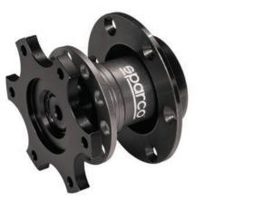
In aluminum with CNC milled steel toothed core. Quick release hub for 6-hole steering wheels with mounting on specific vehicle hub.
