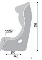
HOMOLOGATION: FIA 8855-1999 MATERIAL: CARBON-KEVLAR PRE-PREG HRS: NO WEIGHT (GR): SHELL: 5300 / SEAT: 6000
