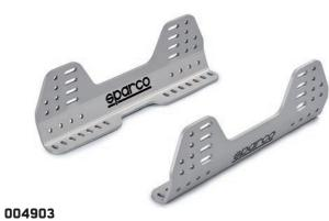
Longitudinal distance between holes 290 mm. Max length 415 mm. Simple mounting in the car with more than 25 positions. 6 mm anodized aluminium.
