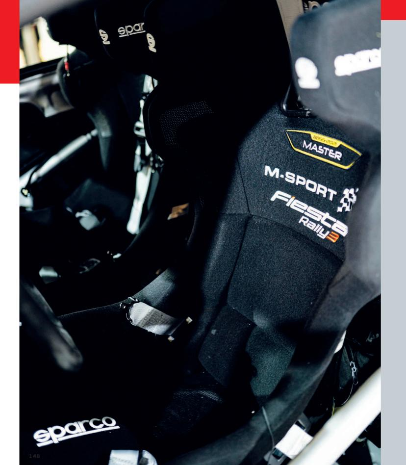
HOMOLOGATION: FIA 8855-2021 MATERIAL: FIBERGLASS HRS: YES WEIGHT (GR): SHELL: 12000 / SEAT: 14900
