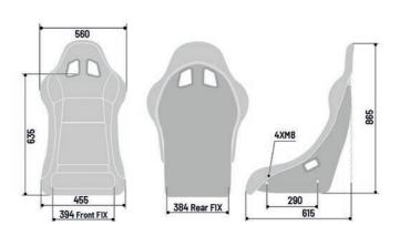
HOMOLOGATION: FIA 8855-1999 MATERIAL: TUBULAR FRAME HRS: NO WEIGHT (GR): SHELL SPRINT: 7940 / SEAT SPRINT: 9700
